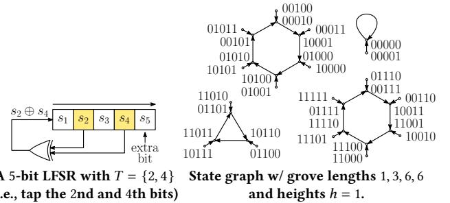
(a) **Strategy A:** add one useless bit to the LFSR in Figure 3a. The same type of growth from cycles to groves occurs starting from Figure 3b.
