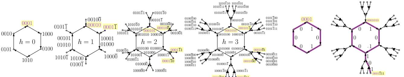
(a) Groves of height  $h = 0, 1, 2, 3$  are generated by the 4-bit LFSR  $x^4 + x^2 + 1$  with  $h$  useless bits. The  $h = 0$  grove is a cycle in Figure 3a, while the  $h = 1$  grove is in Figure 4a. Each grove has one highlighted state with prefix 0001 on its cycle; it is a cyclic substring of its cycle's sequence 000101. The other highlighted states differ in a suffix of length  $\leq h$  (with the first differing bit overlined).
