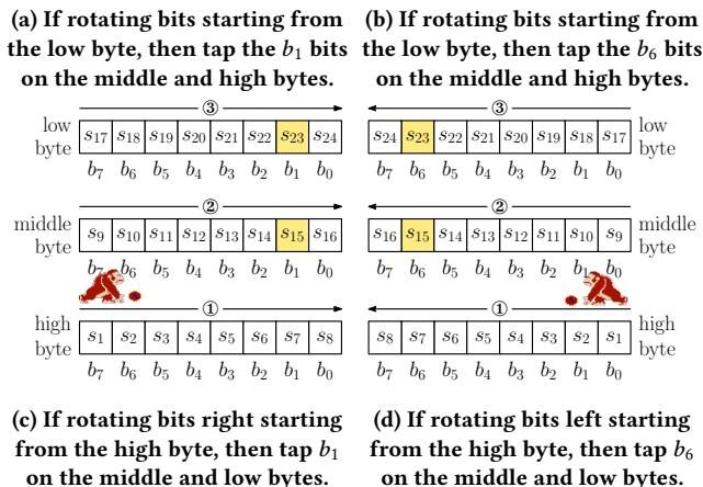
**Figure 7:** Four correct ways to implement a 23-bit LFSR with taps  $\{15, 23\}$  on an 8-bit CPU like the MOS 6502. The implementations can shift each byte's bits to the right or left, and can perform the three shifts starting from the lowest or highest addressed byte.
