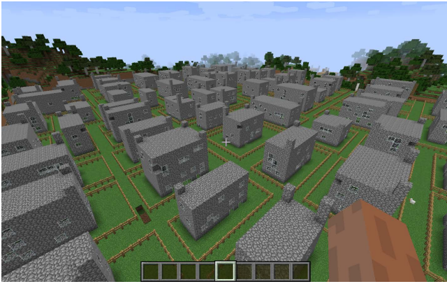
Figure 5: A settlement generated using the sample agent provided in the competition framework. This example uses Binary Space Partitioning to divide the terrain into lots, and a Cellular Automaton to generate the buildings.
